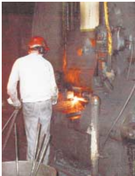
Veteran hammerman, Paul Johnson, operates one of the drop hammers at Lakeview Forge.
